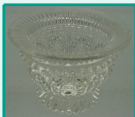
Blown, probably by the Robinet process, cracked off and then placed on a pontil, and the rim tooled and flared out; colorless, intricate pattern of arches and small dots, rough pontil mark; 2 7/8" dia. x 2 1/2" high .
